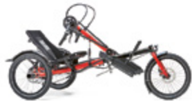
KETTWIESEL HANDBIKE Special Trike with Hand Cranks
